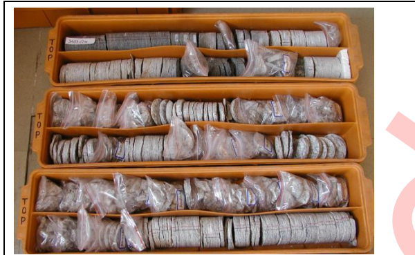
图3 CCSD-1井3478-3524m井段的岩心片化现象 Figure 3 Disced cores obtained in 3478-3524m section of CCSD-1 well
